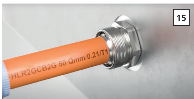
Screw the lower part into the housing with a torque of 25 Nm. Insert the cable with the contact sleeve as far as it will go.
