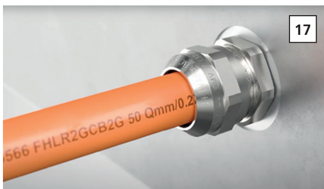
Tighten the pressure nut to fully stop, with a torque of 20 Nm.
